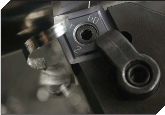
3F Geometry machining ATI 6-4™ Titanium Alloy
