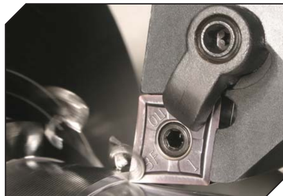
3F Geometry machining ATI 718 Plus® Nickel Alloy
